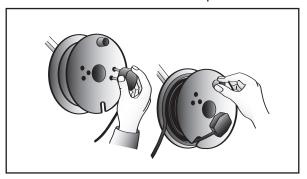
To recoil the hose: Place the steam plate end of the hose into the side aperture of the spool and then wind the hose onto the spool.
